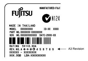
Figure 7.2 Display of disk drive revision number
